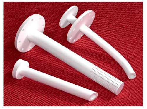
Molded from heavy-wall, Virgin PTFE tubing, MFP Seals designs and manufactures both Dip Tubes and Spargers (Aerators) for applications where metallic tubing may have an adverse reaction with other materials or liquids. MFP Seals T1000, Virgin PTFE material remains inert and will not contaminate other compounds or liquids that it comes in contact with. We design our PTFE Dip Tubes and Spargers with a threaded tube and flange, that when assembled is also back-welded to ensure rigidity.
